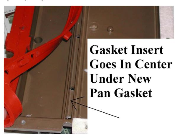
To prevent this from occurring an insert/filler was developed constructed of the same Red RTV silicone material as the gasket that fills this gap. Production gaskets have now been changed to add this insert and re-designed gasket.
